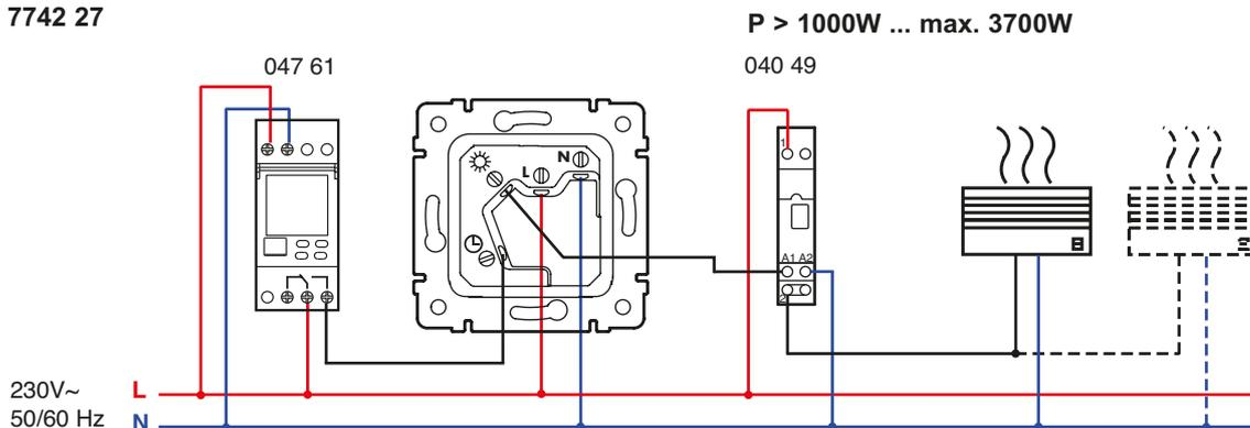
• **Attention:** Distribution voltage to be connected cophasally to thermo regulator and remote control. Installation and assembly may only be effected by an expert!
